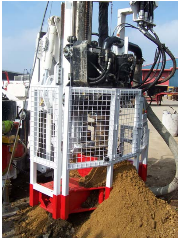
Guarded with front mounted interlocked gates
